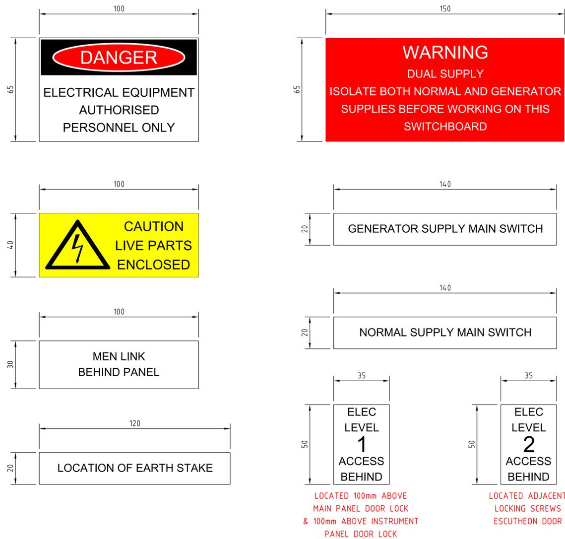
LOCATED 100mm ABOVE MAIN PANEL DOOR LOCK & 100mm ABOVE INSTRUMENT PANEL DOOR LOCK
