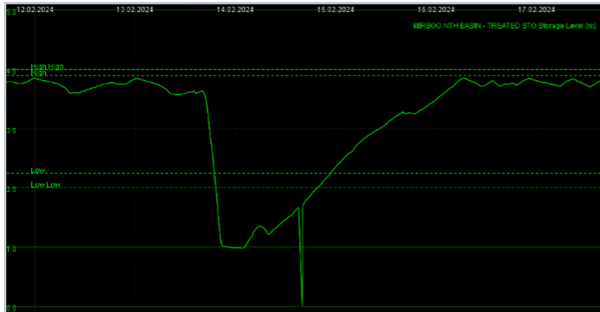
Figure 11: Mirboo North water storage basin level showing a sudden drop caused by the mains break.
