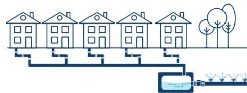
Figure 3-4 Cluster system servicing more than one property. If scale is > 5,000 L/day on any day the system requires EPA approval for existing and proposed systems.
